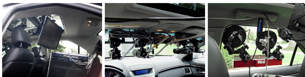
Figure 2.4: The RoadLAB in-vehicle laboratory: a) (left): on-board computer and LCD screen, b) (center): dual stereo front visual sensors, c) (right): side stereo visual sensors.
