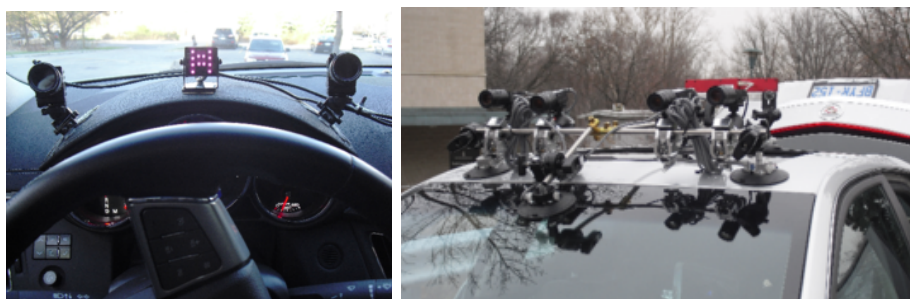
Figure 5.1: Physical configuration a) (left): Remote eye-tracking system, and b) (right): RoadLAB stereoscopic vision system
