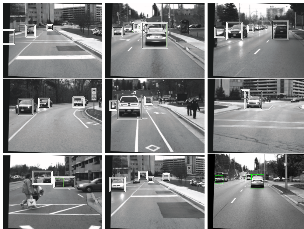
Figure 4.4: Examples of detection results for various frames, including errors
