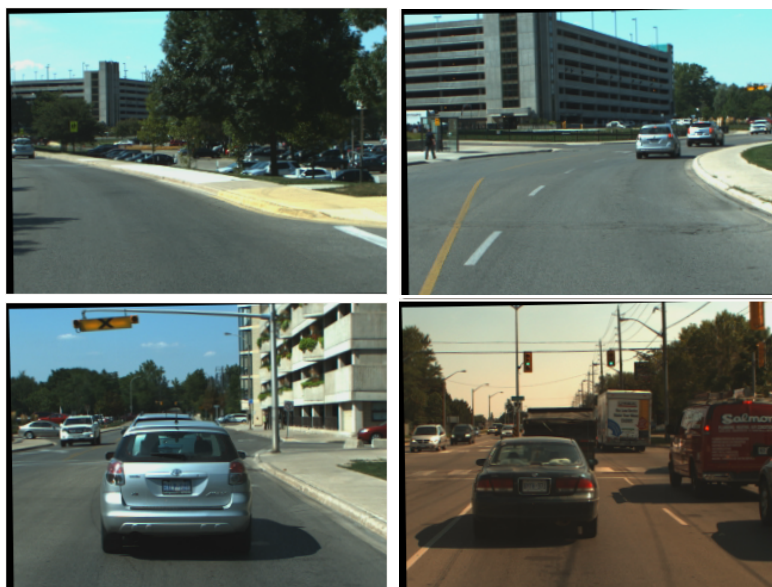
Figure 3.1: Challenges of lane detection: a) (top-left): different curvature and shapes b) (bottom-left): vanished lane markers c) (top-right): splitting and merging lanes d) (bottom-right): occlusion and clutter
