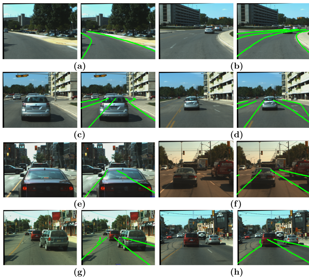
Figure 3.7: Examples of lane detection results a) Out-of-sight lane markers b) Multiple curved lanes c) Occluded lane markers d) Splitting lane e) Urban distractions f) Multiple lanes partially occluded g) Splitting lane and occlusion h) Irregular lane shape
